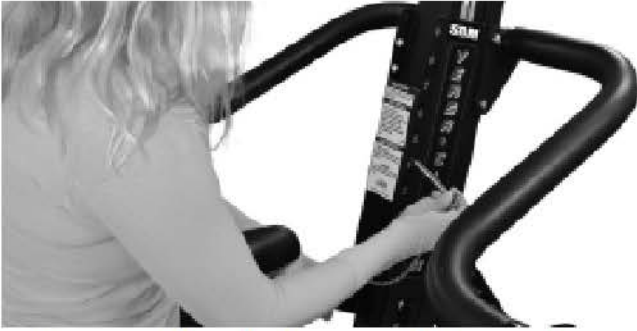
Mounting seat bracket assembly to post.
