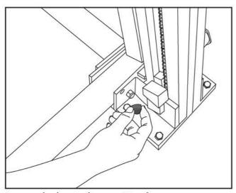
Locate bolts and nuts. Firmly press caps on.
