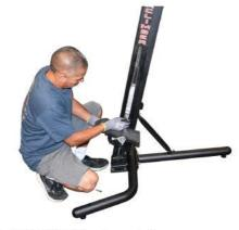
Securely TIGHTEN foot pedals. NOTE: It is recommended to visually inspect foot pedals and tighten bolts every (2) two months and replace pedal shaft every three years.
