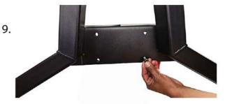
Insert four 3/8 - 1" bolts from the bottom of the machine upwards. Torque wrench setting is 40 lbs.
