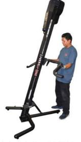
Attach side handrails with (3) three hex head bolts 4 1/4" long and (3) three 3/8" lock nuts. Torque wrench setting is 20 lbs.
