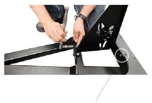
Push two bolts through - do not apply nuts at this time, these two bolts are placed to hold stablizing fin in place before attaching to post. Torque wrench setting is 40 lbs. 6.
