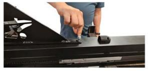
Place 9/16 nut onto post bolt, finger tighten the nut. Once ready to securely tighten, Torque wrench setting is 20 lbs.
