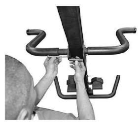
Insert 3" long spacer and FULLY TIGHTEN ALL three bolts and nuts. Torque wrench setting is 20 lbs.
