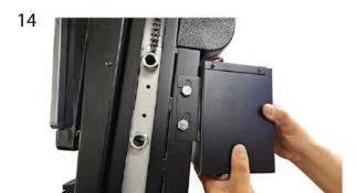
Next attach battery box onto post bolts. Loosen these 2 bolts so as to allow the battery flanges to hook and seat properly onto bolts.
