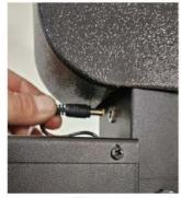
Plug small battery cord into power port as seen here.
