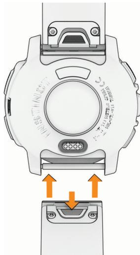
**NOTE:** Make sure the band is secure. The latch should close over the watch pin.
